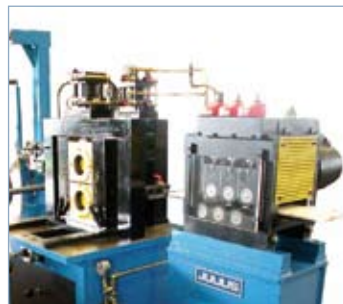
Flat levelling machine type DRAP integrated into strip edge trimming line
