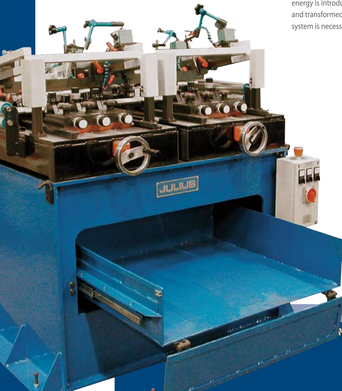
DUO strip edge trimming machine with telescopic swarf box
